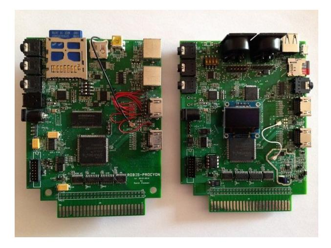
Spartan 6 Xilinx FPGA is a very popular, versatile, inexpensive and yet powerful family of the programmable logic devices. It was selected for its lowest specific cost per logic gate and excellent performance index. This FPGA sports the special dedicated very high speed peripheral interface, which is used by the HDMI standard. This physical interface is called TMDS (Transition Minimized Differential Signalling).
